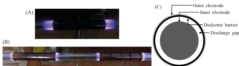
Figure 2. Reactor configuration for one outer electrode (A), two outer electrodes (B), and the cross-section of the reactor (C).
