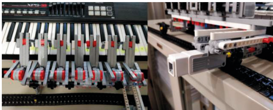
Figure 2. It shows the robotic arm that contains seven large motors (left) and a medium motor (right).
