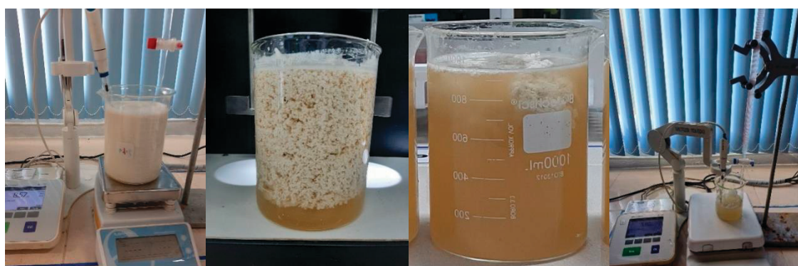
Figure 5. Preparation of skim latex serum and adjustment of alkalinity of serum water with liquid products from pyrolysis at a temperature of 500 °C.
