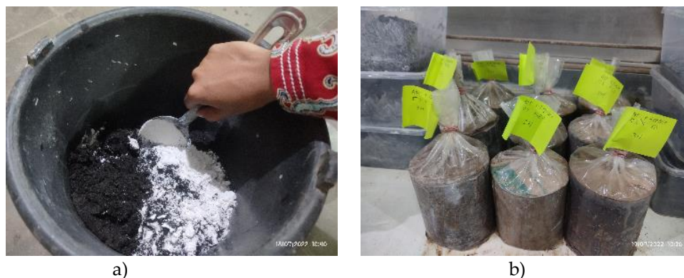
Figure 3 The mixing process for the sand soil stabilization experiment, a) the process of mixing the stabilizing agent and b) Curing the specimen
