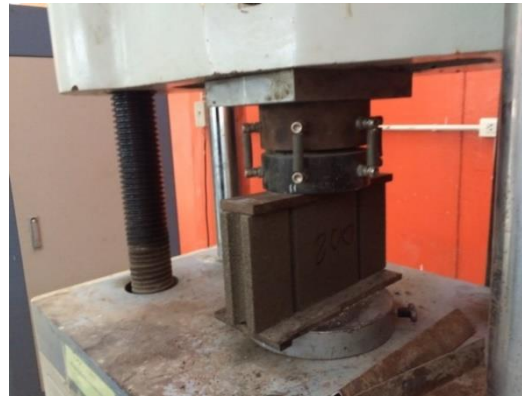
Figure 6. Compressive Strength Test of Hollow concrete blocks.
