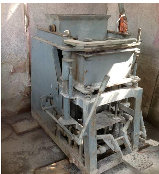
Figure 4. Vibrating hollow concrete blocks compactor.
