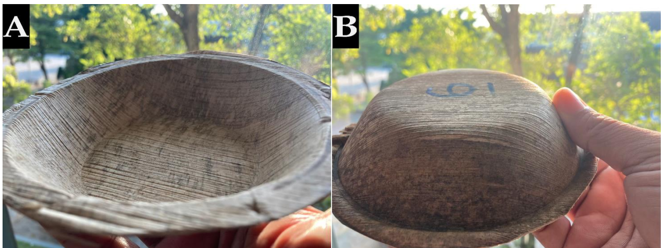
Figure 6. Food plates made from areca nut leaf sheath molded at 160 °C.
