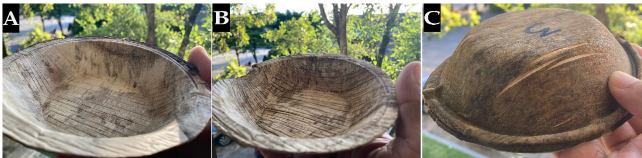
Figure 5. Food plates made from areca nut leaf sheath molded at 150 °C.
