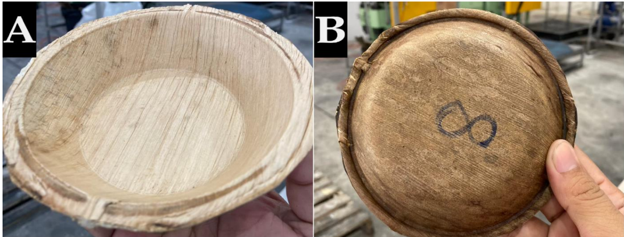
Figure 7. Food plates made from areca nut leaf sheath molded at 170 °C.
