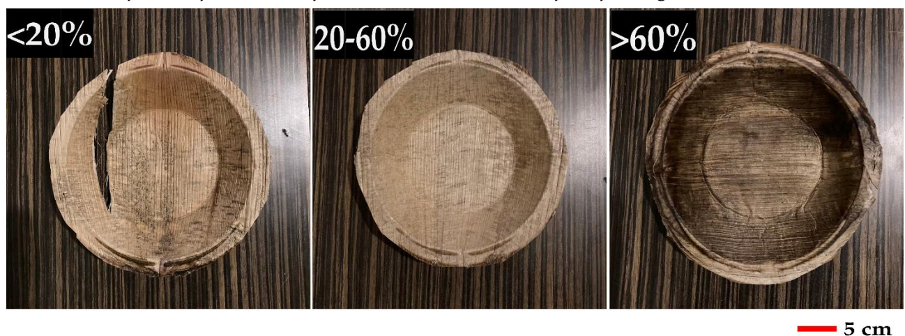
Figure 8. Effect of moisture content on the appearance of food plates made from areca nut leaf sheath.
