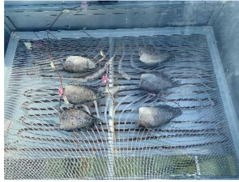
Figure 4. New solar drying cabinet and pulsing heat pipes' placement
