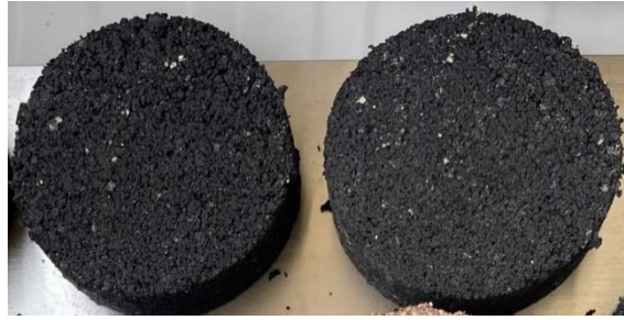
Figure 7(e). Characteristics of fuel briquette obtained from the condition of 67% latex waste sludge mixed with 33% rubber leaf charcoal.
