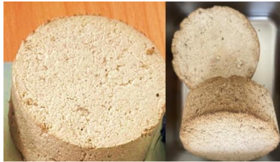
Figure 7(a). Characteristics of fuel briquette obtained from 100% latex waste sludge condition.
