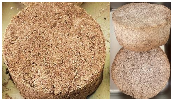
Figure 7(b). Characteristics of fuel briquette obtained from the condition of 83% latex waste sludge mixed with 17% raw rubber leaves.
