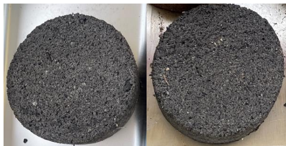
Figure 7(d). Characteristics of fuel briquette obtained from the condition of 83% latex waste sludge mixed with 17% rubber leaf charcoal.
