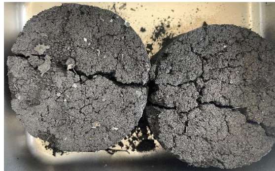
Figure 7(f). Characteristics of fuel briquette obtained from the condition of 67% latex waste sludge charcoal mixed with 33% rubber leaf charcoal.
