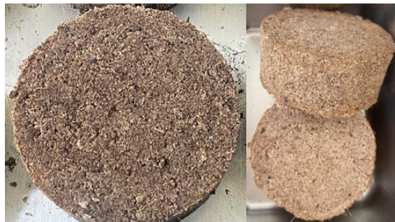
Figure 7(c). Characteristics of fuel briquette obtained from the condition of 67% latex waste sludge mixed with 33% raw rubber leaves.
