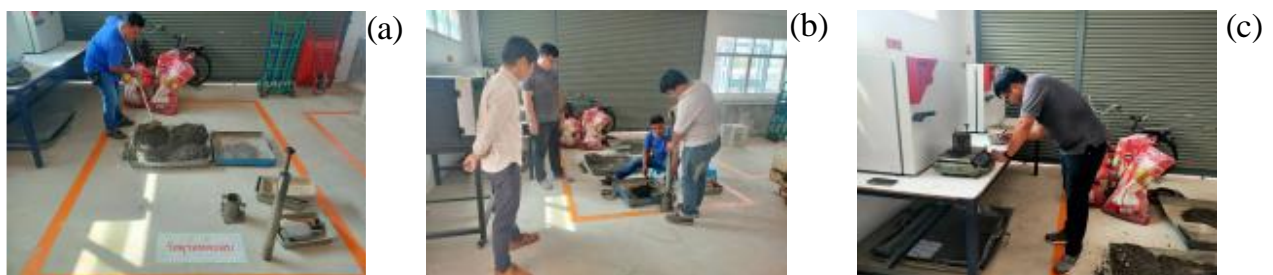
Figure 4. Compaction test (a) preparation of soil and RAP (b) soil compaction test in operation (c) taking measurements for density calculation
