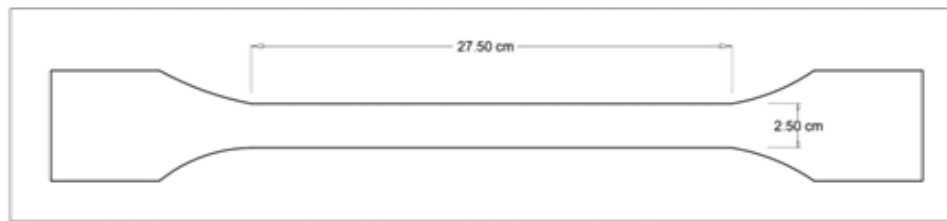
Figure 1. Dimensions of a tensile sampling
