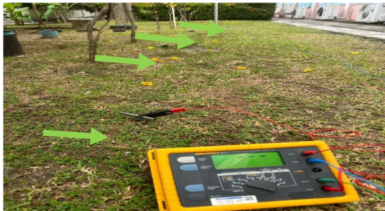
Figure 4. Wenner four-pin method for soil resistance measurement.
