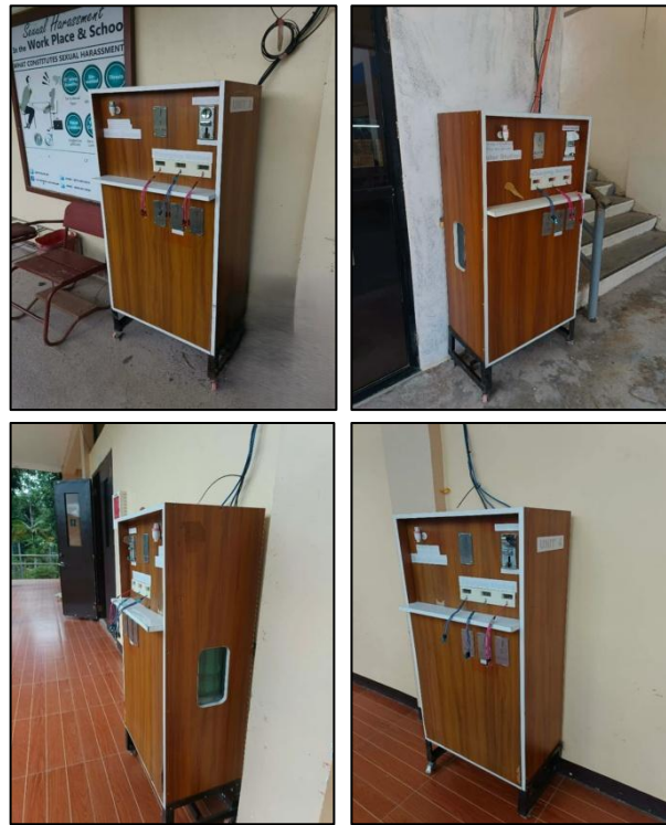
Figure 4. Actual Campus Set-up of Solar-Powered Vendo Machine
