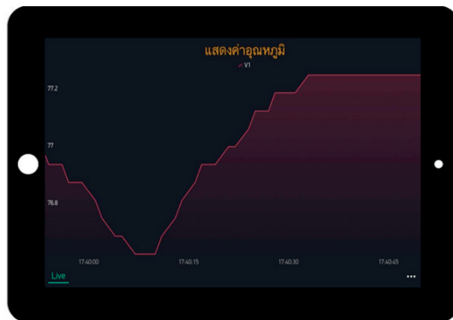
Figure 4. Thermal analysis graph for changing state of matter with smart learning media displayed through the IoT system displayed with the Blynk application on a smart device
