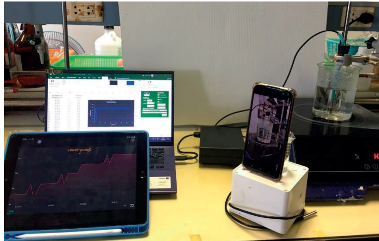
Figure 3. An experimental set for studying the changing state of matter with smart learning media displayed through the IoT system for smart-lab
