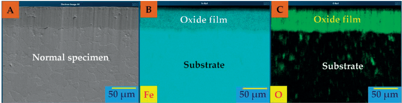
Figure 9. EDS mapping of cross-section's surface normal specimen (A) SEM micrograph (B) iron (C) oxygen
