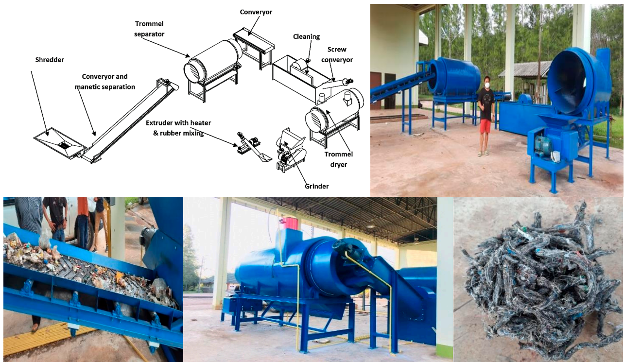
Figure 2. A prototype system for the production of refuse-derived fuel (RDF-5) at a production capacity of 800 kg/day
