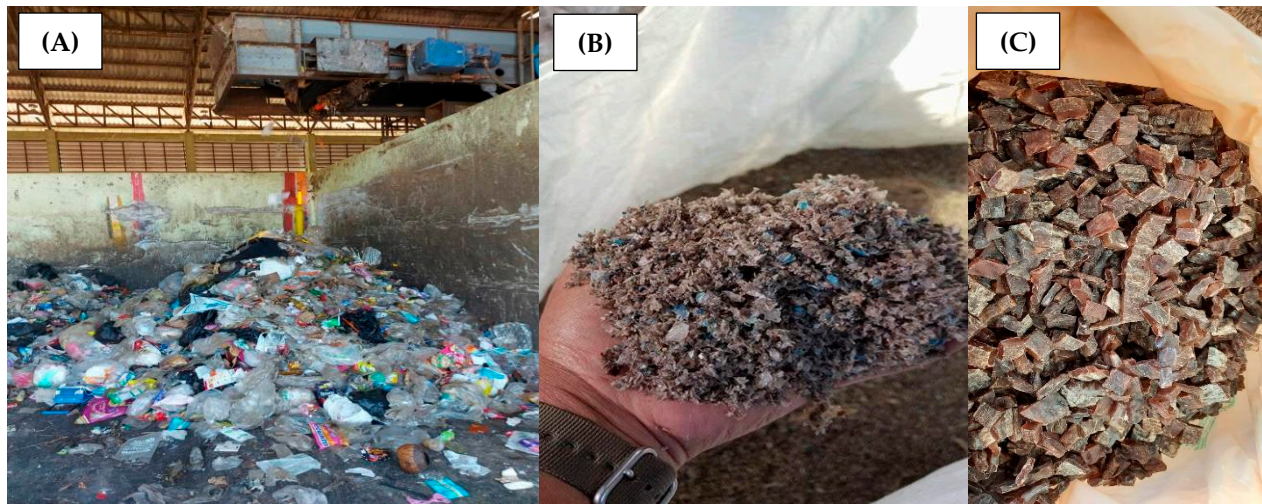
Figure 1. Materials used in the experiment; (A) Municipal solid waste, (B) Ground solid waste, and (C) Ground natural rubber
