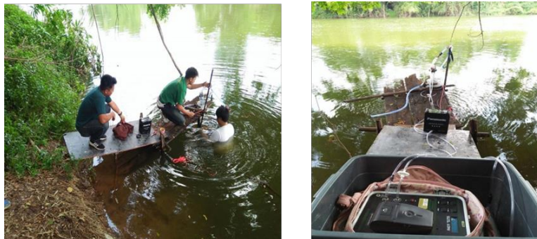
Figure 3. The stations continuously measurement of radon concentration in Site 1 Ban Tha Ruea, Khuean Ubonrat Sub-district along the lower Nam Phong River.
