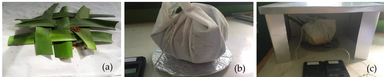
Figure 4. (a) Herbal preparations, (b) Wrapping the Pot, (c) Measuring the temperature inside and outside the pot
