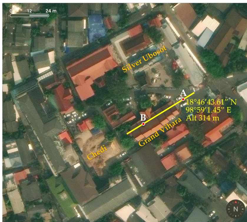
Figure 1. A satellite image of Sri Suphan Temple's Grand Vihara, with a yellow line indicating its axis. Points A and B are designated for a theodolite setup along the temple's axis. Map data: © OpenStreetMap contributors.
