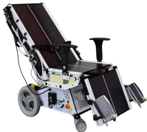
Figure 3. Positions of stretcher cum wheelchair for radiographic purposes driven by electronic motor. The base is made from stainless steel, the body made from 3 carbon fiber plates: the low extremity, the body, and the head part. The lower part of all fiber carbon plates has a slot for the image receptor. The motor driver can adjust the position of the image receptor.
