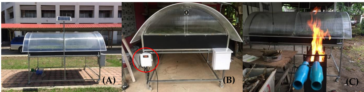
Figure 4. Prototype of KLs drying technology: A) Using solar energy, B) Temperature control system, and C) Using heat from biomass
