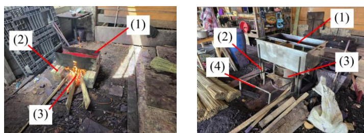
Figure 2. Dyeing of krajood using a biomass stove. (a) traditional stove (b) improve biomass stove
