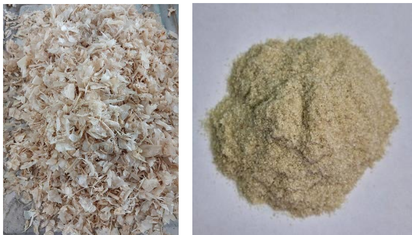
Figure 1. Chitin (left) and chitosan (right) purified from white shrimp shells after chemical extraction
