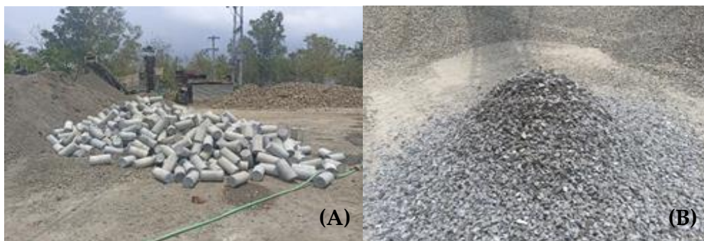
Figure 3. Concrete cylinder waste: A) Before crushing, B) After crushing.
