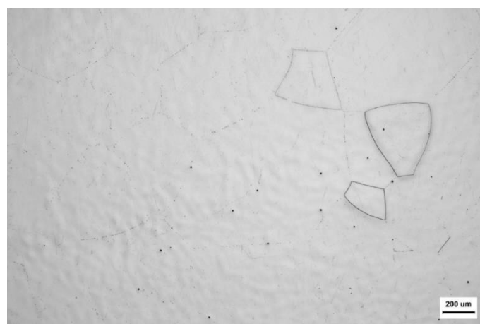
Figure 6. Microstructure of the Ti-45Nb titanium alloy sample.
