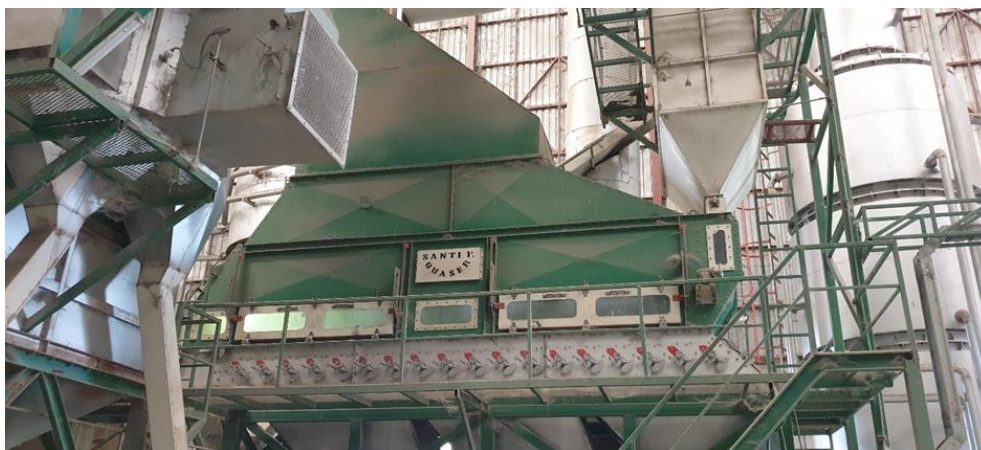
Figure 2. Components of the Fluidized bed (Ref.Tor Thaicha Roen Rice Mill Co., Ltd.).
