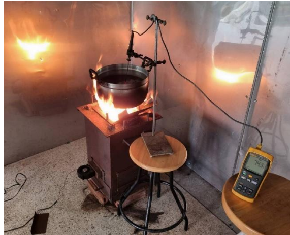
Figure 4. Performance evaluation of TLUD biomass stove with the WBT method
