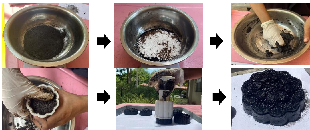
Figure 3. Molding of tea waste–reinforced molded charcoal products using a mooncake mold.
