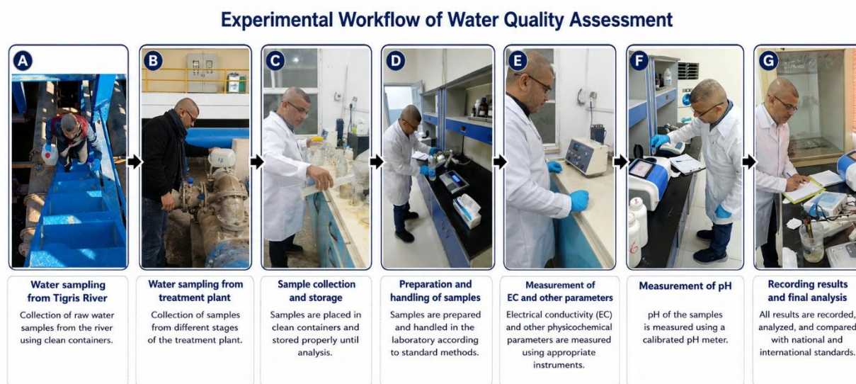
Figure 1. Experimental workflow of water sampling and physicochemical analysis in the Al-Aziziyah–Al-Hafariya water treatment system.
